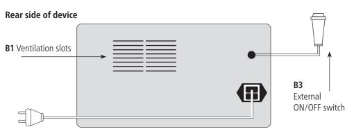
Mains connection ~ 230 V 50/60 Hz with fuse protection 2 x T 1.6A H 250 V
