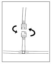
When removing the expansion, loosen it on the hose coupling.
