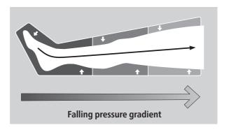
The air chambers remain filled with air until the uppermost chamber has reached the corresponding pressure. After that, the pressure escapes from all air chambers simultaneously and begins the pump-up cycle anew after a pause period. The intermittent compression has an impact on the individual tissue layers and the blood and lymphatic vessels they contain.
